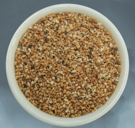
Boiler Bed Material
